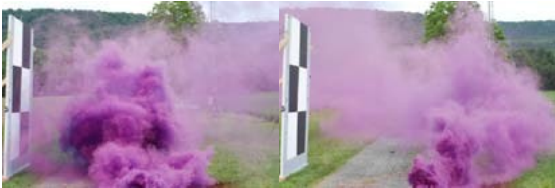
Figure 5-18 Emission of a passive substance 15 s (left) and 55 s (right) after the release. Side view (above) and view from behind (below) (from Long et al., 2010)
